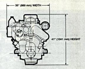
For complete dimensional information, refer to installation drawing 2SA256 for model 1042-5000 and 2SA260 for model 1042-3000
